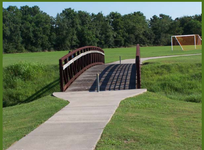
Bollards or other barriers help to keep motorized vehicles off trails but must not impede trail access for persons with disabilities.
